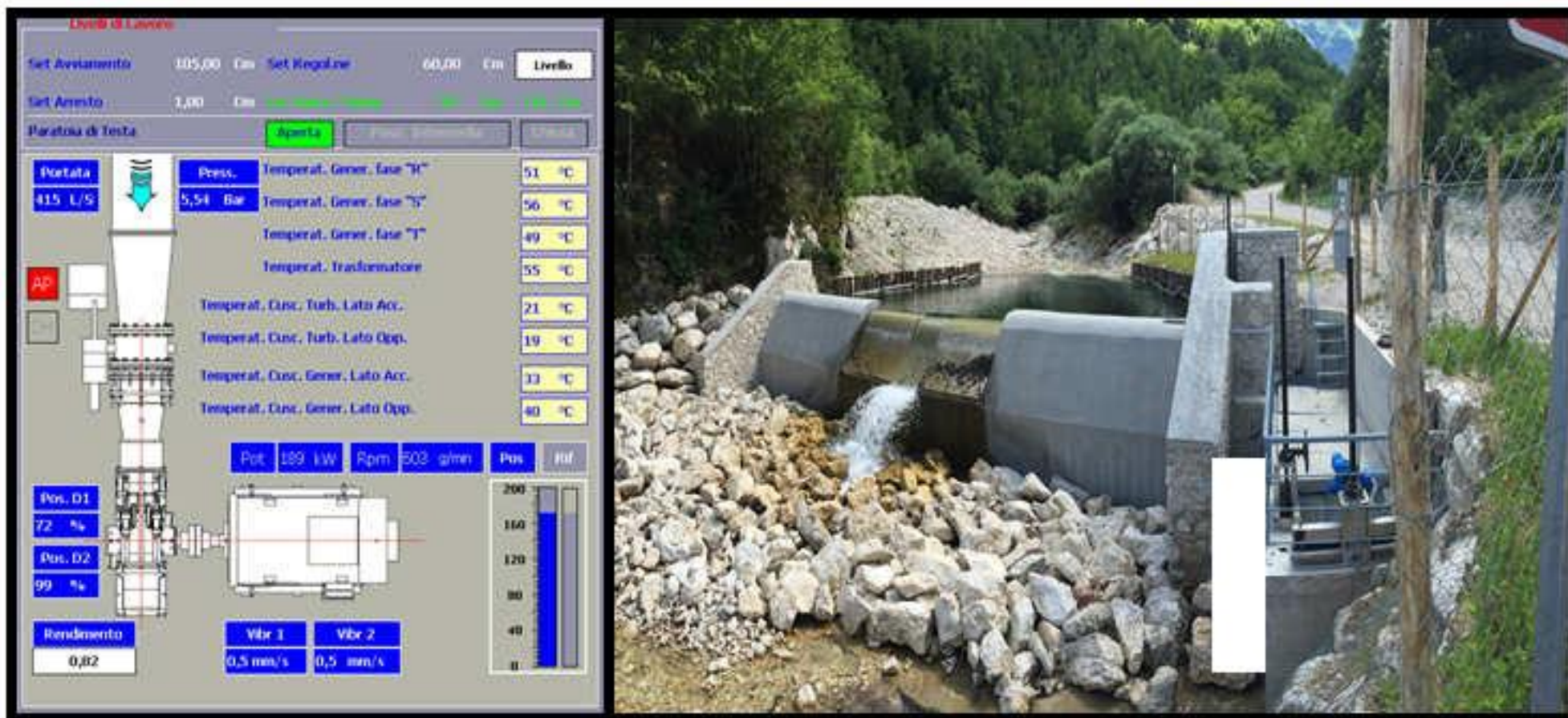
Example of control system: real time measurement, data and image acquisition
